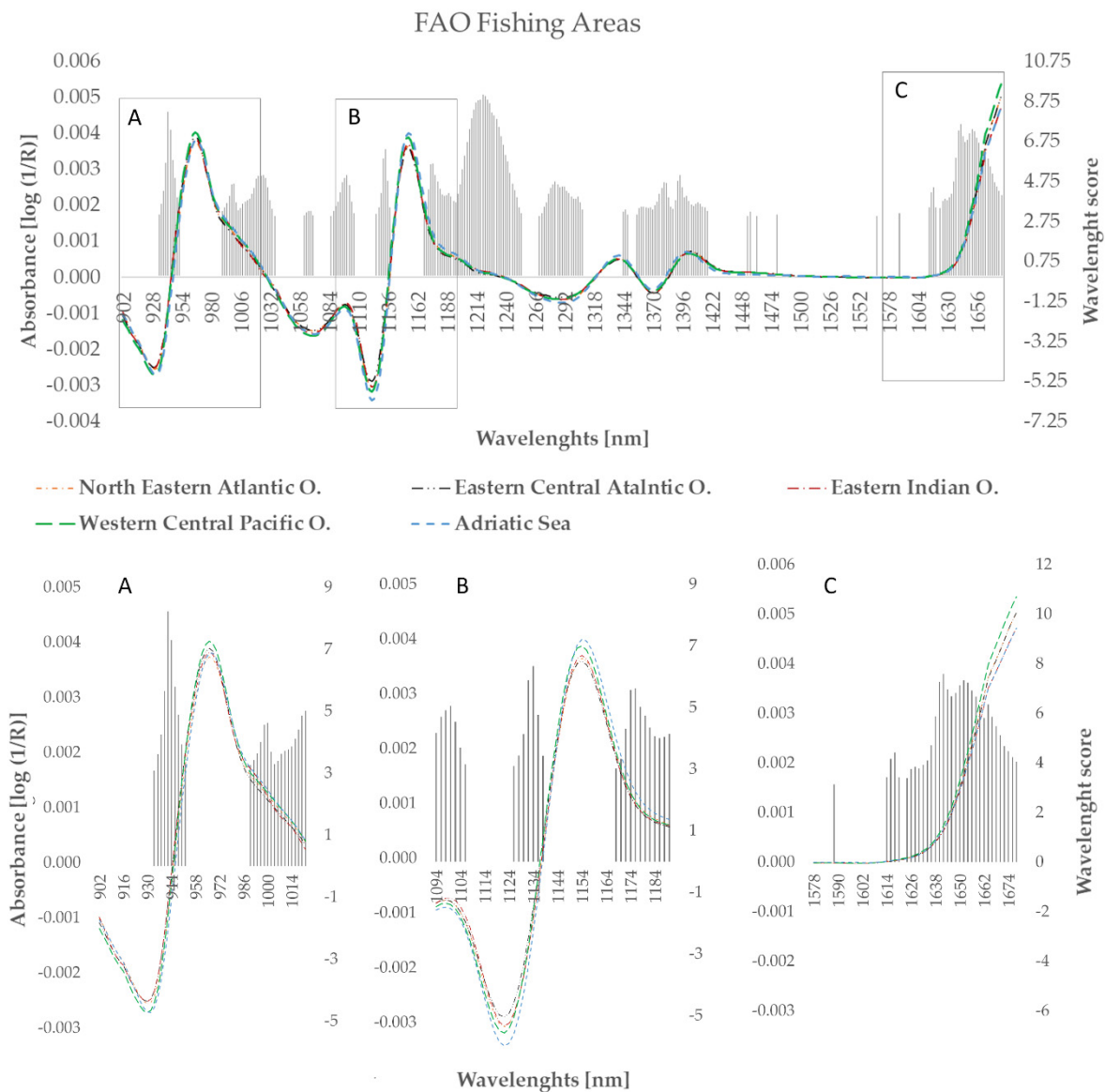
Figure 1. The mean NIR absorbance curves after standard normal variate, detrending, smoothing and the second derivative treatment and the most informative wavelengths selected by random forest (in grey) for predicting origin of FAO fishing area in cuttlefish. Magnification of spectra ranges where the differences in absorbance were detected (A) (902–1022 nm), (B) (1094–1190 nm), and (C) (1578–1678 nm).
